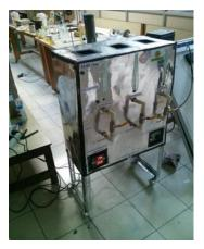
The process, known as trans-esterification, converts carboxylic acid ester into a different carboxylic acid ester. Apart from the waste cooking oil, it requires water, alcohol and a catalyst.
